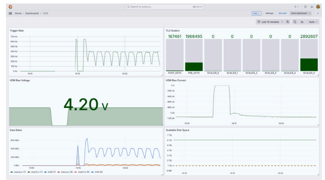
Fig. 18. Example of a Grafana Dashboard displaying telemetry data of a Constellation . Shown are trigger rate information emitted by a satellite controlling the AIDA-2020 TLU [38], voltage and current information from a Keithley 2410 power supply satellite, and data rate and disk space information from a Constellation receiver satellite.
